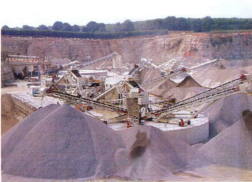
The new 350 tonnes/h Powerscreen washing plant at Hermitage Quarry, near Maidstone, Kent.
