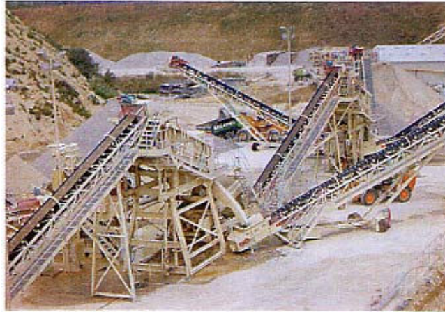
Sharp and soft sand and 20mm, 14mm, 10mm and 6mm graded products are now recovered from the hassock
