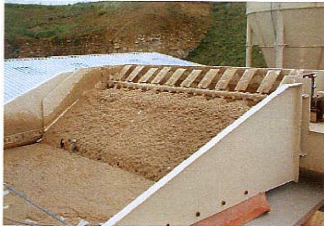
Thickened silt being fed on to one of the multi-roll belt presses
